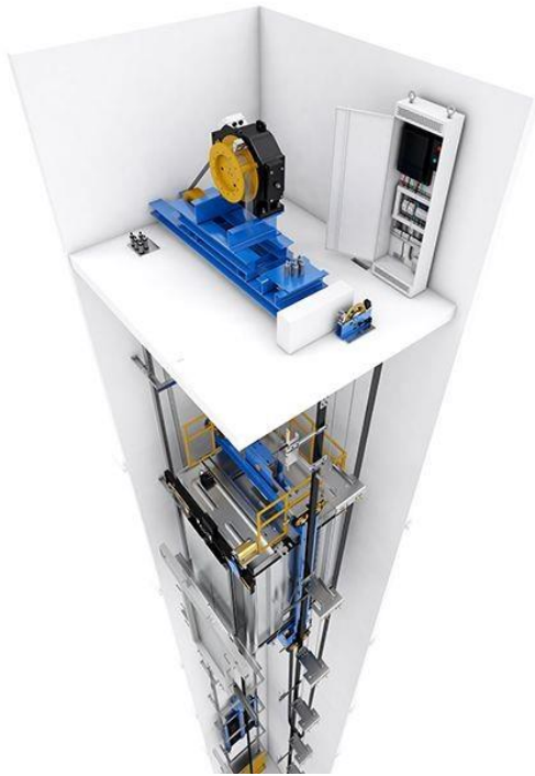
Machine room elevators (MR)
